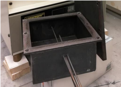
Cooling water for the liquid collector (optional)
